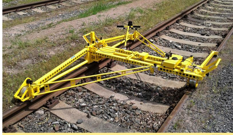
Track Recording Trolley for track geometry
